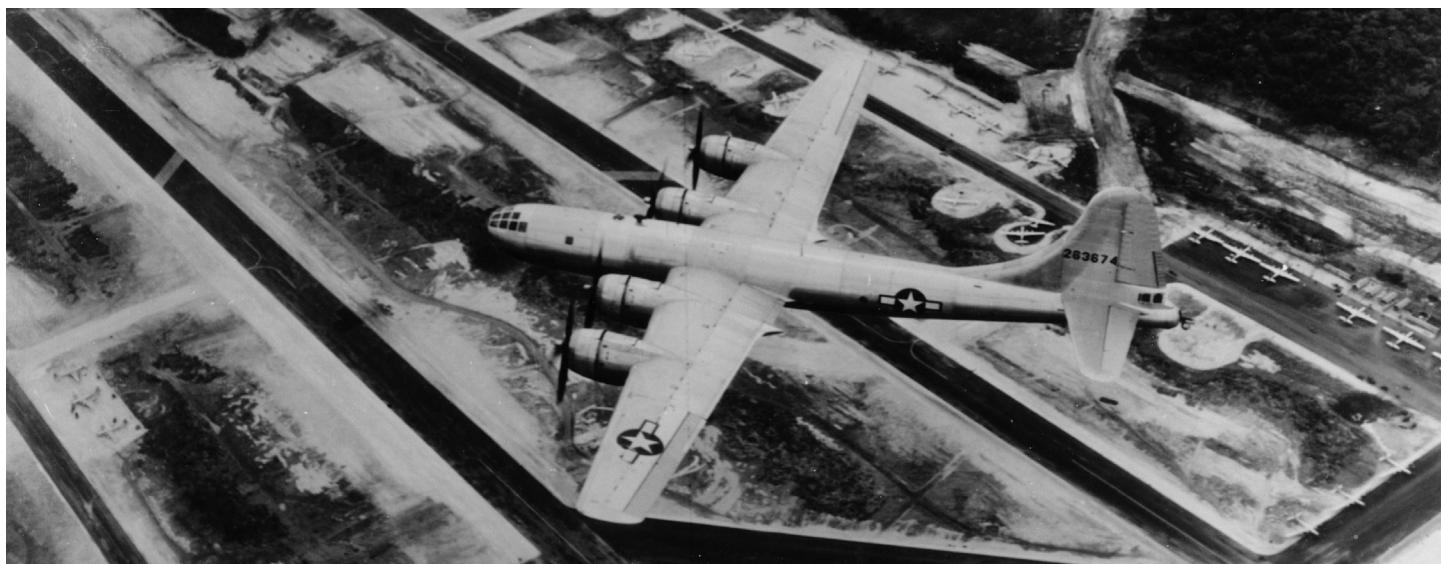
A B-29, the only WWII aircraft with a pressurized cabin, flying over Guam. ( The National WWII Museum, 2010.216.358 )
